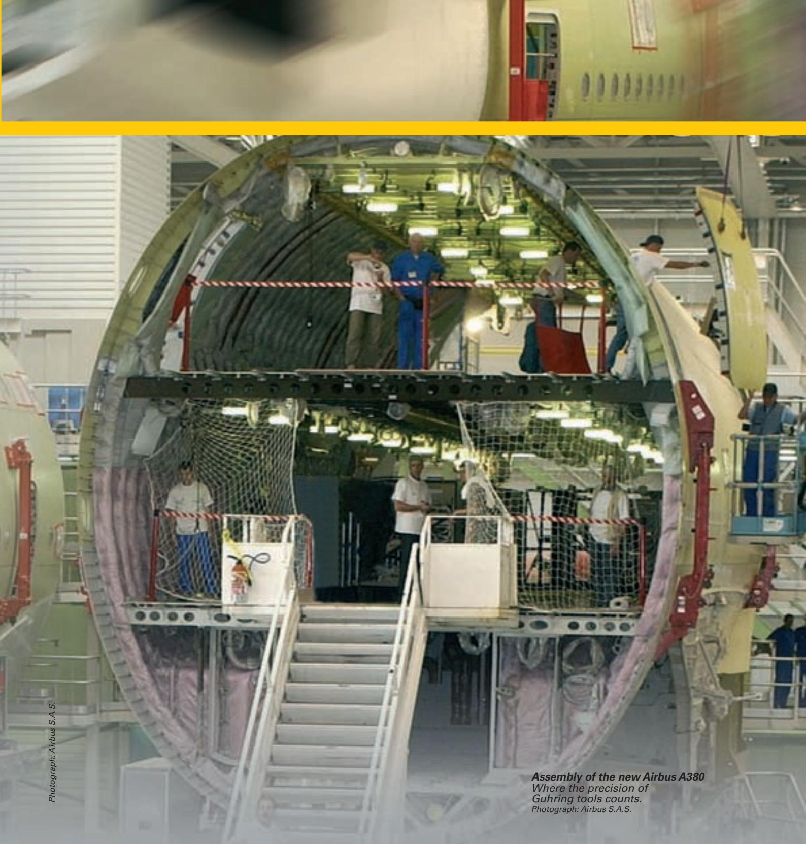
**Assembly of the new Airbus A380**
