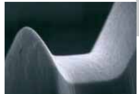
Optimised surface of a Guhring Profile fluteless tap
