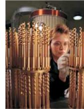
to promote optimum coating uniformity and thickness. Properly cleaned and sorted, the tools and parts are then placed in the coating chamber. We monitor the coating process closely so that the structural integrity and the geometry of the tool or part remains intact.
