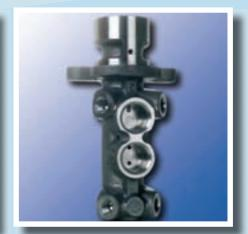
Safety components: Drilling and reaming a master brake cylinder
