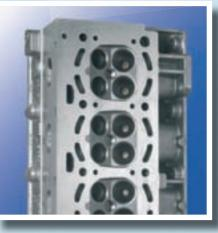
**Demanding:** Complete machining of cylinder head
