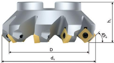
Axial rake angle  $\gamma_a = +5^\circ$
