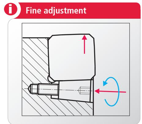
Fine adjustment using a tapered screw
