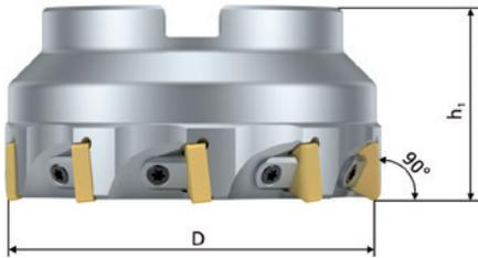
Axial rake angle  $\gamma_a = -6^\circ$
