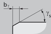
Chamfer width  $w_\gamma$  in 1/100 mm and angle  $\gamma_s$  without degree symbol
